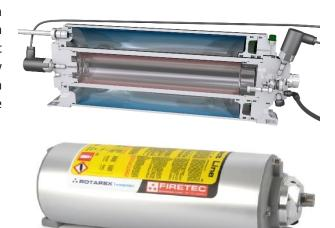
The FireDETEC® Compact Line System can be equipped with a special heat-sensitive tube, the FireDETEC® sensor tubing. The FireDETEC® sensor tubing is connected to the Compact Line and pressurized with 16 bar nitrogen gas. It reacts to fire and extreme temperatures and must be installed in the fire hazard area. It bursts at approximately 120°C. The bursting of the FireDETEC® sensor tubing triggers the fire suppression process.
